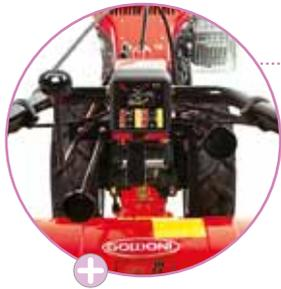
+ Device that prevents the reverse gear from being engaged when the PTO is used for cultivating work.
