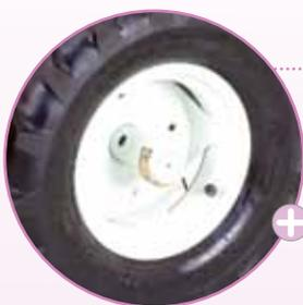
+ The external width of the wheels and the track width are adjustable. The adjustments adapt the machine to specialized crops.
