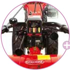
⊕ Device that prevents the reverse gear from being engaged when the PTO is used for cultivating work.
