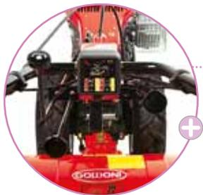
+ Device that prevents the reverse gear from being engaged when the PTO is used for cultivating work.
