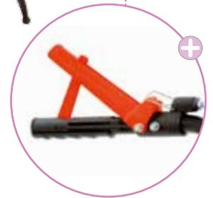
⊕ "GEARSTOP" does not turn the engine off but it locks the transmission and the PTO, in case of release of the handlebar grip.
